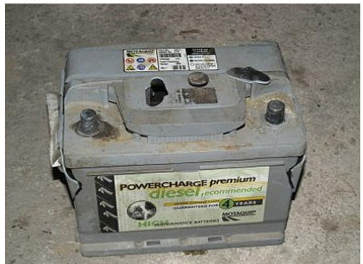
in an internal explosion. The force can burst the plastic casing or blow the top off the battery, spraying acid and casing fragments. An explosion in one cell may ignite the combustible gas mixture in remaining cells. In a poorly ventilated area, connecting or disconnecting a closed circuit (such as a load or an operating charger) directly to the battery terminals may cause an explosion as the sparks produced ignite the gas mixtures vented from the cells.
